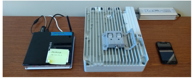
Figure 2: dLTE prototype components: A mini-computer, commercial eNodeB, and off-the-shelf handset
